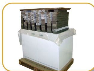
Actual photo during Cabinet Load Testing
