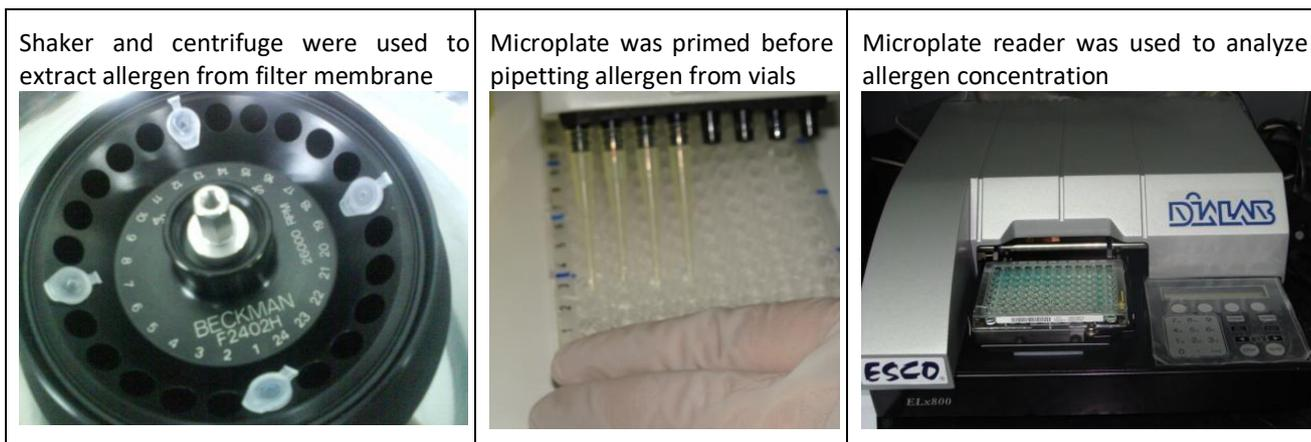
Operator protection efficiency was calculated by comparing the amount of allergen captured by the cassettes worn by the operator against the allergen sampled on top of dirty cages.
