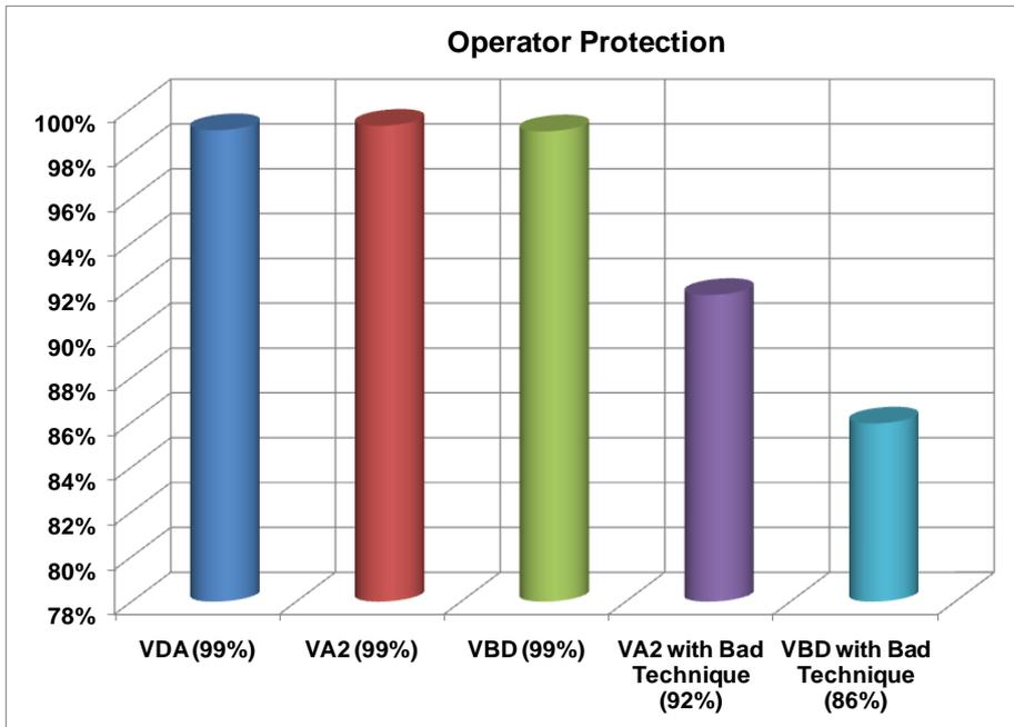
1. All three tested cabinets (VDA, VA2, VBD) have same high operator protection level of 99% when operated using good technique.
