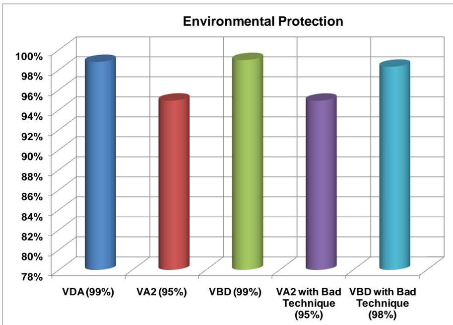
4. The VDA and VBD have high degree environment protection of 99% because unlike VA2, they are equipped with activated carbon filters that help the ULPA filters to further absorb the allergens.
