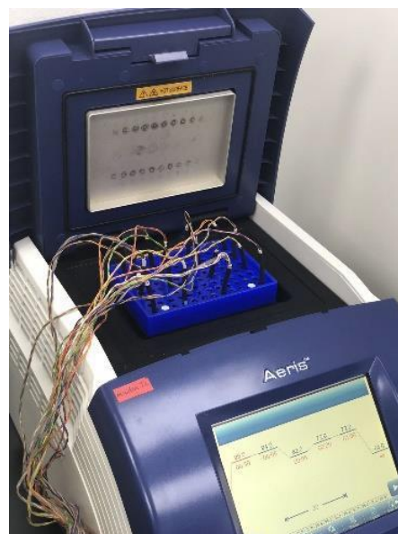
Figure 2. Testing temperature uniformity of the thermal cycler
